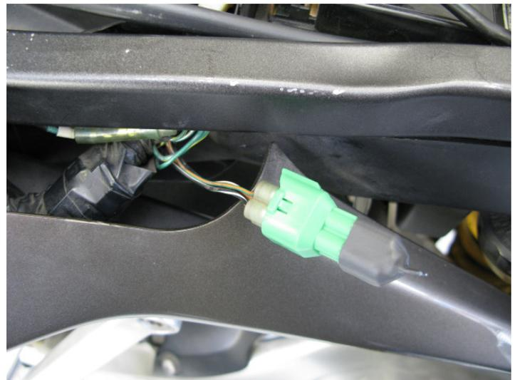
3. Place control unit in the tail compartment and route the fuel and coil harnesses' main connectors up into the compartment from the rider seat area so that the fuel harness is running along the left of the battery and the coil harness is running along the right side of the battery. Connect the harnesses to the control unit.
