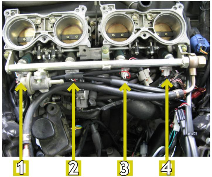
7. Locate the large grey connector on the right side of the fuel rail. There is a **red/yellow** wire that runs between this connector and the blue TPS connector; crimp the supplied skotchlok connector onto this wire and connect the Bazzaz TPS connector.
