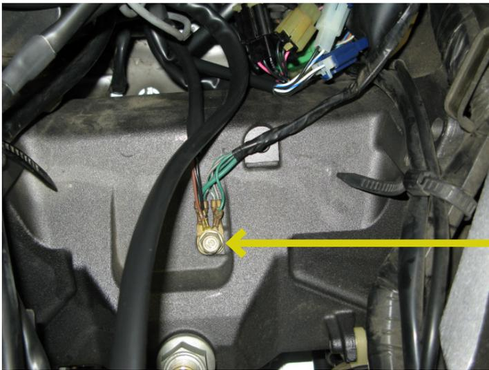
10. Locate a suitable chassis ground to attach the Bazzaz fuel harness ground lug.
