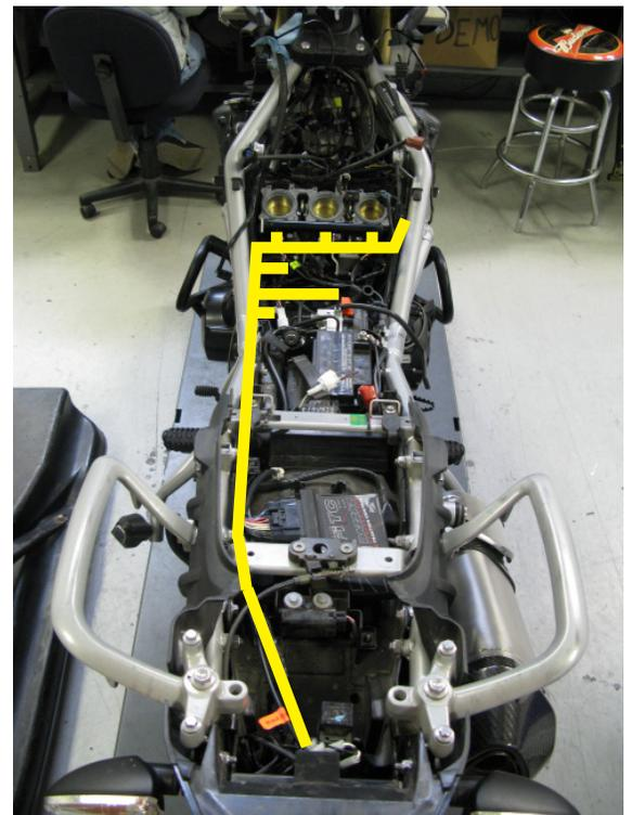
4. Locate the factory speed & neutral connectors (black connectors) found where the subframe joins the frame on the left side of the bike. Disconnect the connectors. Connect the Bazzaz speed & neutral connectors of the Bazzaz fuel harness inline with the factory connectors.
