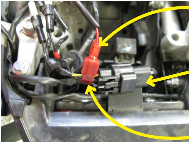
Bazzaz +12V switched power connector (red connector with with red wire)
