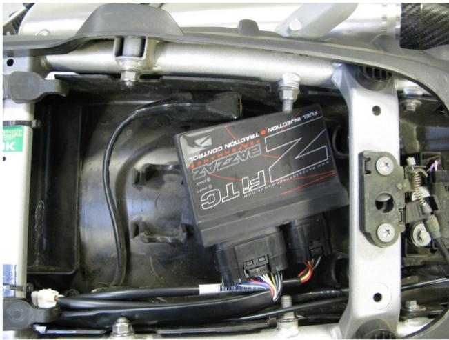
3. Connect the main connector of the Bazzaz fuel harness into the control unit and begin routing the fuel harness towards the front of the motorcycle. Continue routing the harness under the support bar and along the left side of the frame.
