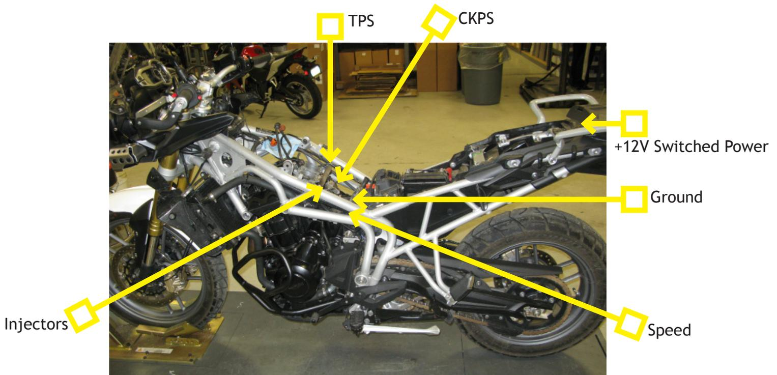
2. Place the control unit in the tail section of the motorcycle, under the passenger seat, and secure it using the supplied Velcro patch.
