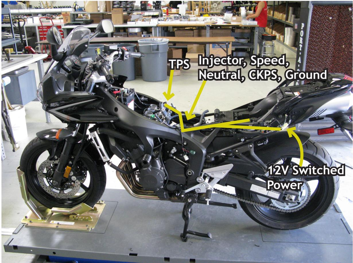
3. Route the Bazzaz +12V switched lead back towards the taillight following the factory harness on the left side of the bike. Pull back the harness sheathing to expose the wires of the factory harness of the tail light connector and crimp a supplied scotch lok connector onto the **blue wire**. Insert the Bazzaz +12V switched power connector (**red wire**) (orange tag) into the scotchlok.
