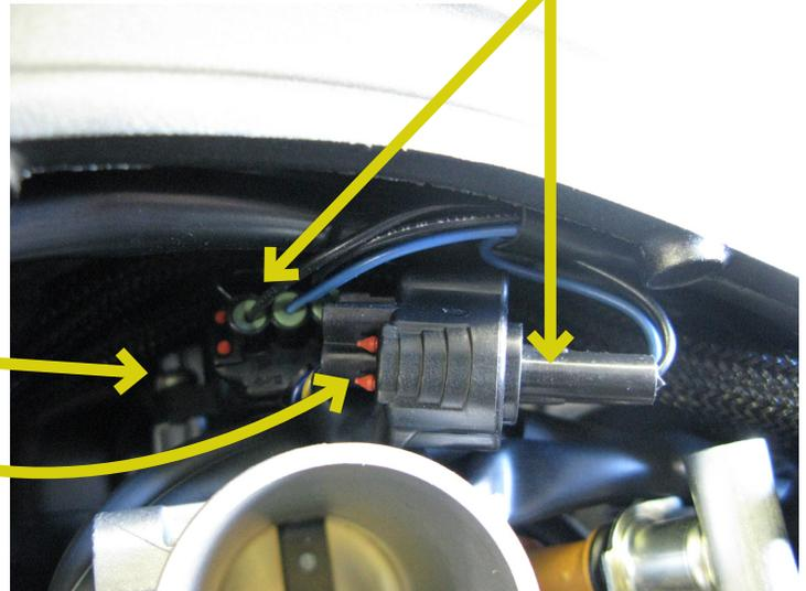
10. Disconnect the factory O2 sensor (black connector) found near Injector and speed sensor connectors. **Note: If not disconnected the factory ECU will continue to make map changes.**
