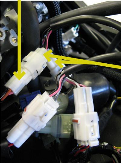
5. Locate speed sensor connectors (middle of engine compartment in rubber boot with other connectors) and install corresponding Bazzaz connectors inline with factory harness.
