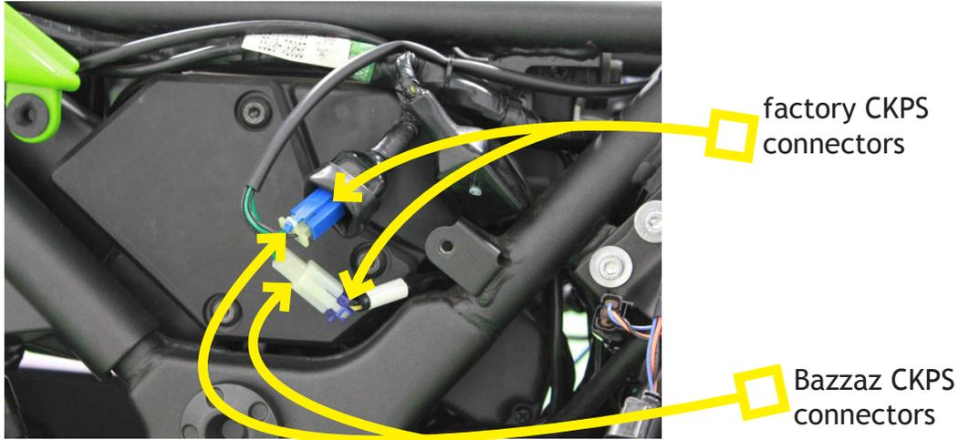
10(B). Locate the black factory CKPS connectors which are found on the left side of the air box and disconnect them. Connect the Bazzaz CKPS connectors in-line with the factory connectors.
