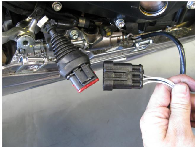
11. Now connect the main connector of the Bazzaz **COIL HARNESS** to the control unit and route the harness up the left side of the motorcycle. Remove the bolts on the factory ECU mounting bracket and pull it back to gain access to the coil connectors. Disconnect each factory coil connector and plug the corresponding Bazzaz **COIL** connectors in-line with the factory connectors. Replace the bolts and ECU mounting bracket.
