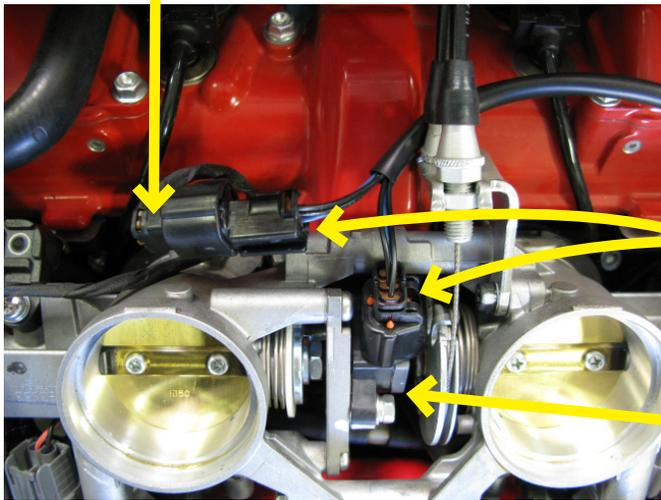
9. Route the remaining fuel harness up the right side of the throttle bodies and around the front, to the factory Throttle Position Sensor (TPS). Disconnect the factory TPS connector from the sensor and connect the Bazzaz **TPS** connectors in-line with the factory sensor and connector.
