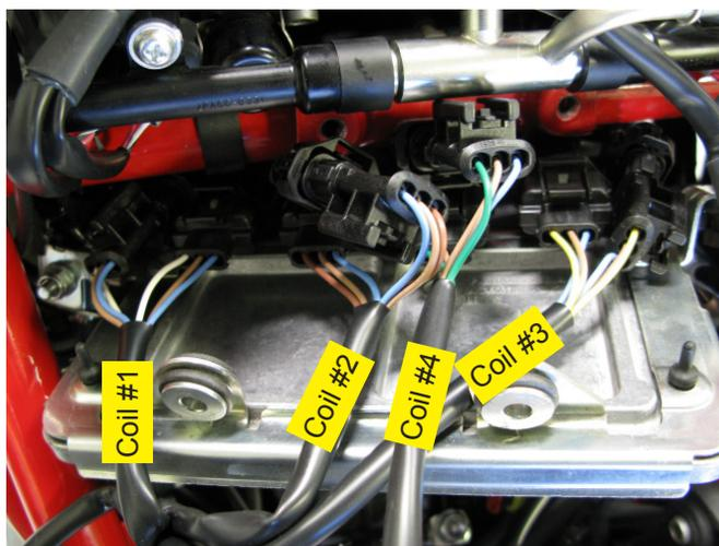
*Bazzaz coil connectors plugged in-line with the factory coil connectors. Factory coil connectors cannot be seen in the photo.*
