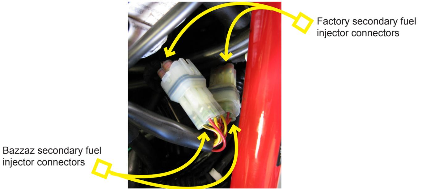
7. Beginning on the right side (which is injector 4), disconnect the factory injector connectors from the injectors and plug the Bazzaz **INJECTOR CONNECTORS** in-line between each factory connector and injector (Bazzaz connector leads are labeled *cylinder 1-4*).
