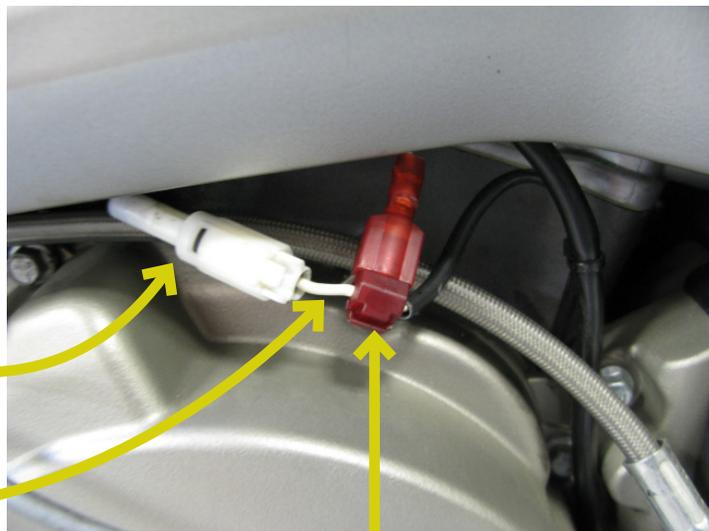
10. Route the Bazzaz speed connector down the right side of the engine and to the top of the right side case cover. Locate the section of the factory harness leading from the factory speed sensor, located on the right rear of the transmission. Cut the factory harness sheathing open to expose the wire and crimp a supplied Scotchlok onto the **gray/white** wire.
